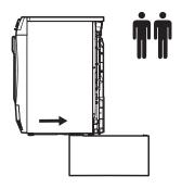
**8.** Move the Pedestal/Appliance assembly to its permanent location. Use a spirit level to check if the assembly is properly leveled. If not leveled, adjust feet to level properly.
